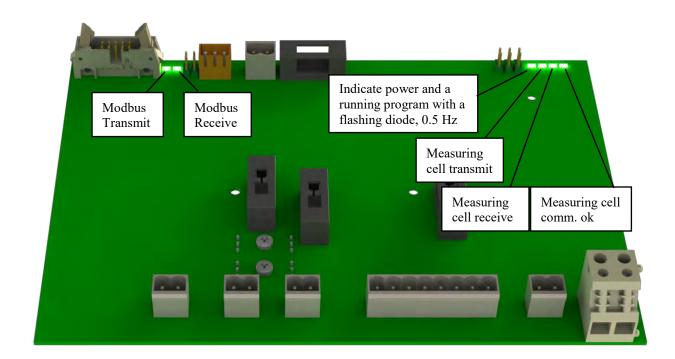
PCB located in the Converting unit, see CTB10003 sheet 3 of 4, Converting Unit page 102, d6.
