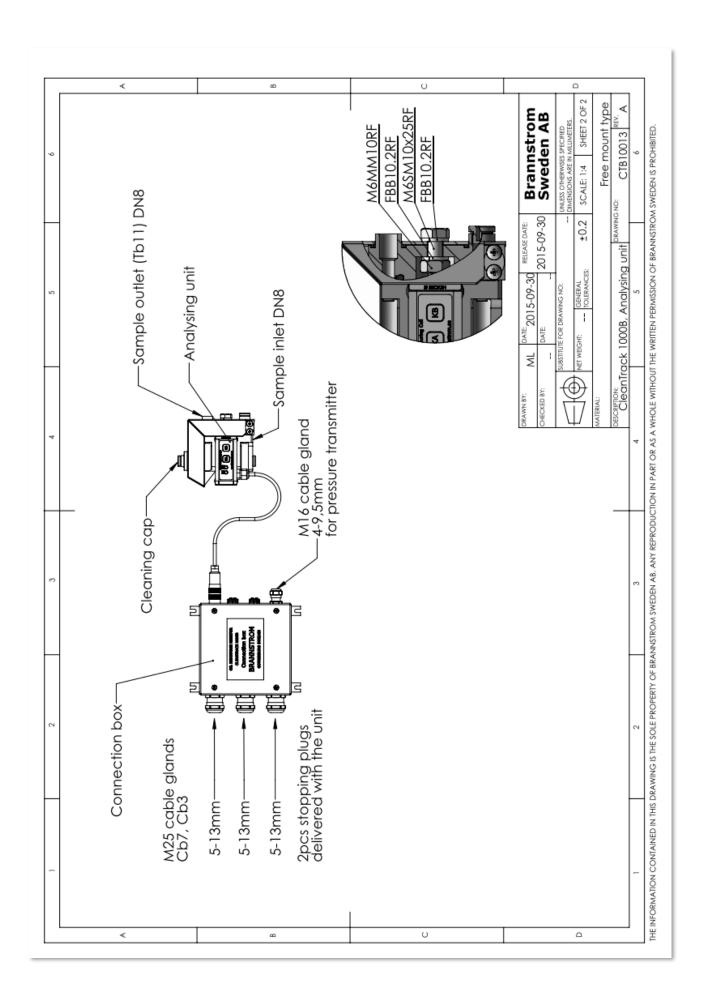
Drawing: CTB10010 sheet 1 of 5, Analyzing unit with air motor sample pump.
