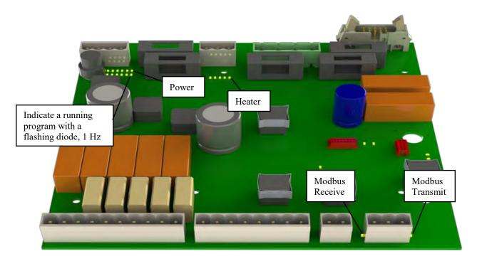
PCB located in the Converting unit, see CTB10003 sheet 4 of 4, Converting Unit page 103, d5.
