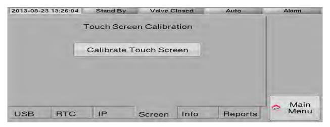
If the touch screen is not in a working condition or behaving strange, a calibration might solve the problem. If it is impossible to maneuver to the touch screen calibration page by using the touch screen itself it is possible to connect a USB mouse to the USB port at the front of the computer unit.
