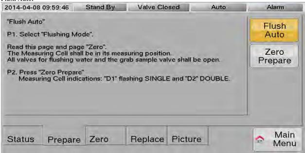
"Flush Manual/Auto" Press this key to toggle between manual flushing and automatic flushing by the "Controlled Water Valve". If "No Controlled Water Valve" is selected in the Setup/Config-page this
