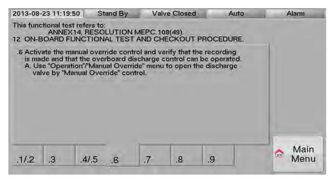
.6 activate the manual override control and verify that a recording is made and that the overboard discharge control can be operated;
