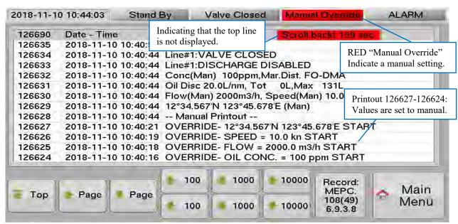
The RED "Scroll back! ### sec" is shown if latest printout is not shown on top line. After 300 seconds (5 minutes) of inactivity, indications will go back to displaying the top line.
