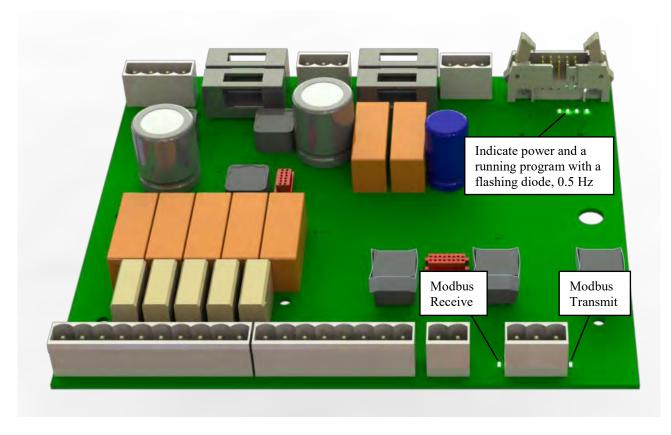
PCB located in the Converting unit, see CTB10003 sheet 3 of 4, Converting Unit page 102, d5.
