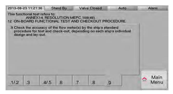
.9 check the accuracy of the flow meter(s), for example by pumping water in a loop where the flow rate may be calculated from the level change in a tank. The check should be made at a flow rate of about 50% of the rated flow of the flow meter.
