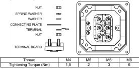
IMPORTANT: <u>Motors with Ex eb terminal box</u> REPLACE THE GASKET (SEAL) IN THE RIGHT POSITION BEFORE CLOSING THE TERMINAL BOX AND SCREW COMPLETELY ALL THE SCREWS.
