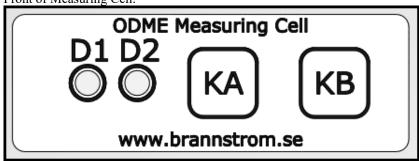
The front of the "Measuring Cell" has two yellow light emitting diodes, "D1" and "D2". It also has 2 touch keys, "KA" and "KB".
