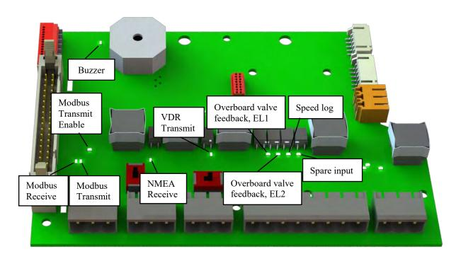
PCB located in the Computer unit, see CTB10001p sheet 3, Computer Unit with open door page 98, d5.
