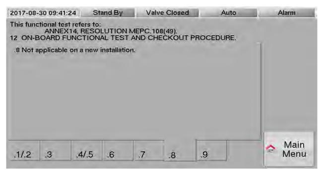
.8 Only in connection to renewal of ship's IOPP Certificate, if a new measuring cell has not been installed, the following should be performed. Start up the system and check the zero and gain settings for the oil content meter in accordance with the manufacturer's operations and technical manual;
