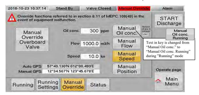
"Manual Override Forcing the Overboard Valve to open.
