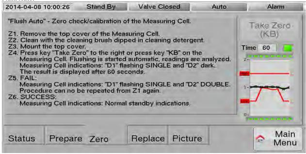
"Take Zero (KB)" Press this key to start Zero Check/Calibration. Reading are analyzed for 60 seconds.
