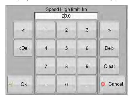
This example shows the "Speed High limit" being set to 20.0 kn.
