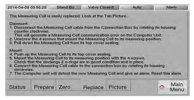
Before replacing the measuring cell, study the chapter 4.10. Measuring Cell Instructions and Replacement page 30.
