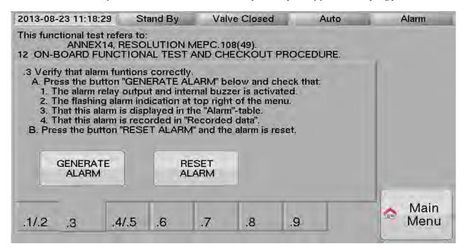
.3 verify that alarms function correctly when a malfunction occurs external to the monitoring system, such as no sample flow, no flow meter signal, power failure, etc.;
