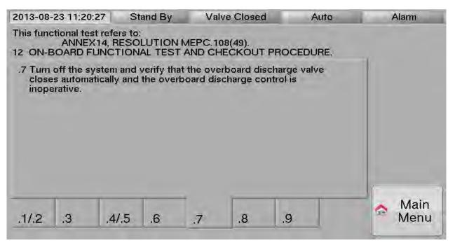
.7 turn off the system and verify that the overboard discharge valve closes automatically or the relevant pumps are stopped and the overboard discharge control is inoperative;
