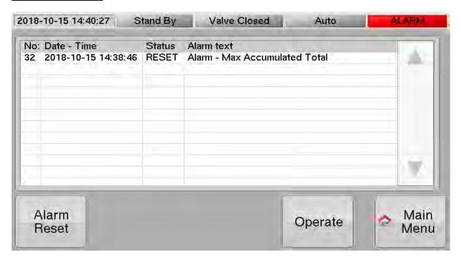
"Alarm Reset" Resetting alarms. Status columns indicates "ACTIVE" for alarm not yet resets and "RESET"
