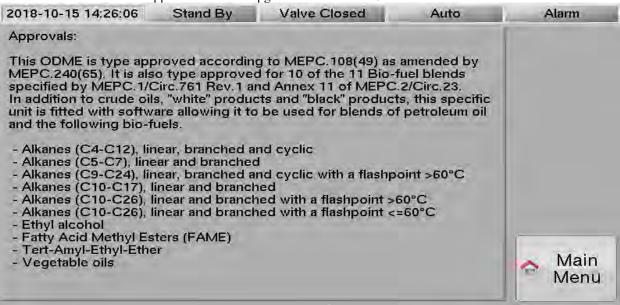
The menu below shows the approvals of a unit approved for the 5 bio-fuels blends according to MEPC.1/Circ.761.
