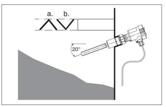
Fig. 3: Horizontal installation
