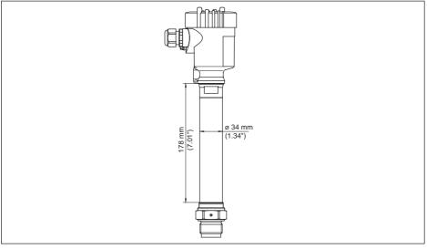
Fig. 33: Temperature adapter
