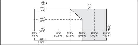
Fig. 30: Ambient temperature - Process temperature
