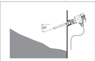
Fig. 4: Horizontal mounting
