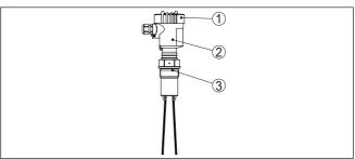
Fig. 1: VEGAWAVE 61 with plastic housing
