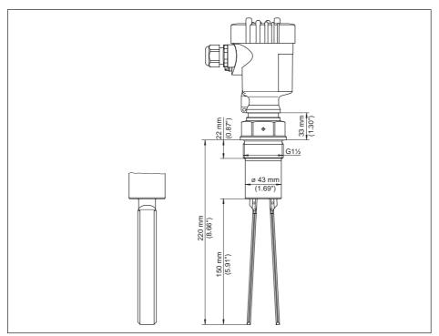
Fig. 32: VEGAWAVE 61, threaded version G11/2 (DIN ISO 228/1)
