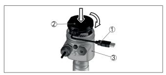
Fig. 39: Connection of the PC directly to the sensor via the interface adapter
