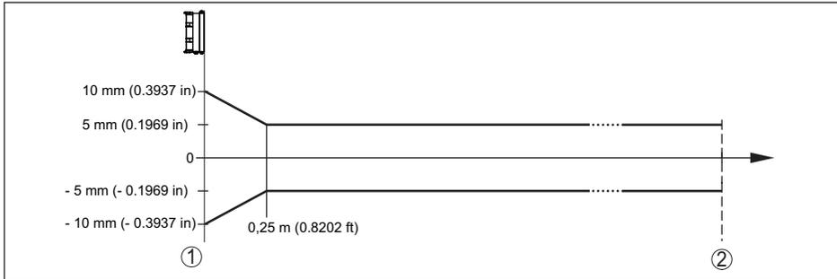
Fig. 17: Deviation under reference conditions
