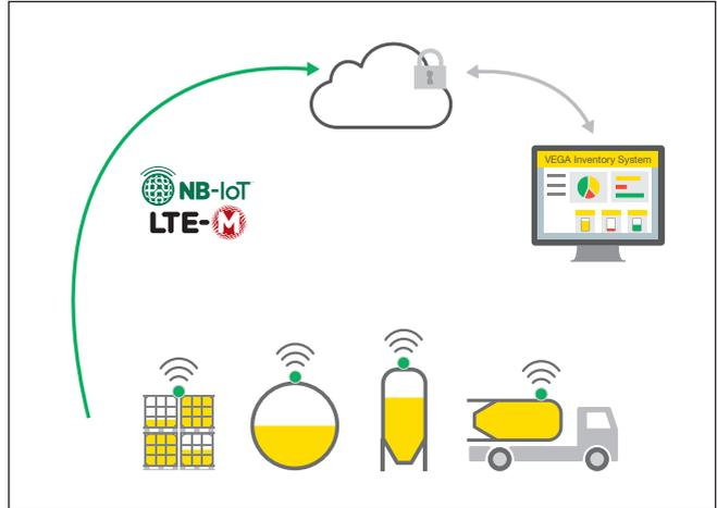
Fig. 3: Wireless measured value transmission via mobile radio
