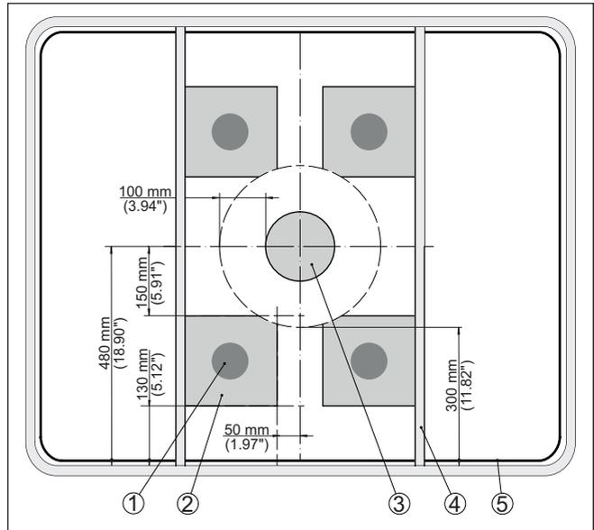
Fig. 5: Mounting position on the tank ceiling
