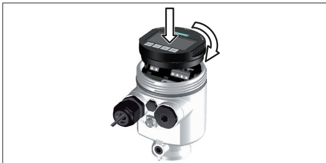
Fig. 21: Installing the display and adjustment module in the electronics compartment of the single chamber housing
