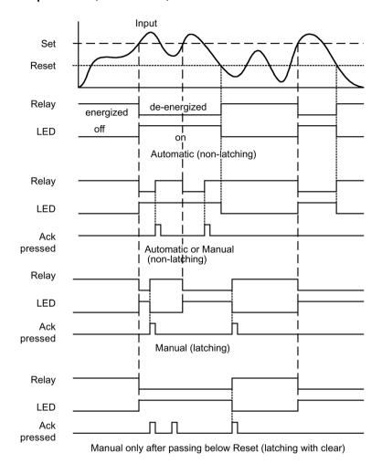
The relay coil is energized in non-alarm condition. In case of a power failure, the relay will go to alarm state.
