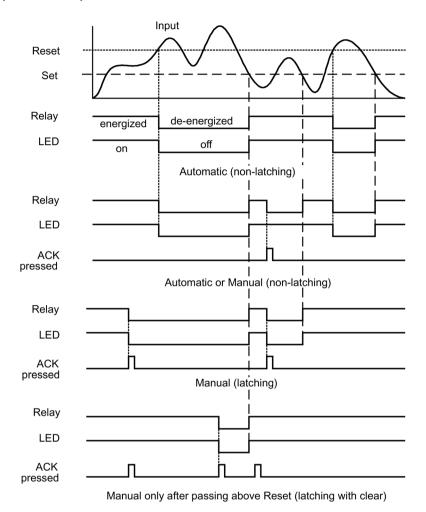
For Manual reset mode, **Enter/Ack** can be pressed at any time to turn off relay. For relay to turn back on, signal must go below setpoint, and then go below it.
