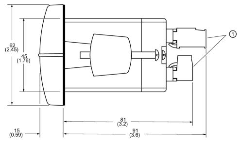
① Screw terminal connector [0.5 Nm (4.5 lb/in) tightening torque]
