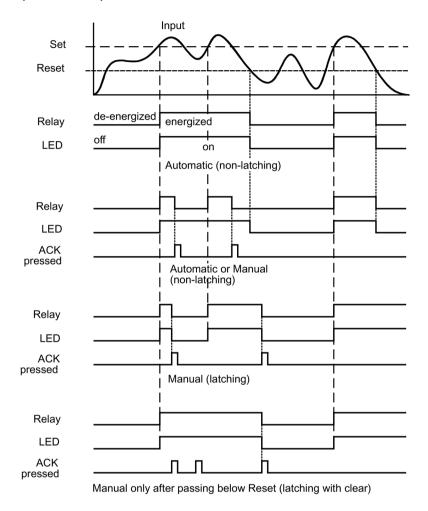
For Manual reset mode, **Enter/Ack** can be pressed at any time to turn off relay. For relay to turn back on, signal must go below setpoint, and then go above it.
