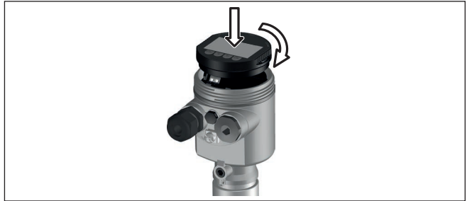
Fig. 29: Installing the display and adjustment module in the electronics compartment of the single chamber housing
