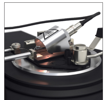
Automatic dip of ignition source and flash detection
