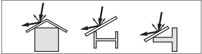
Fig. 13: Cover flat, large-area profiles with deflectors
