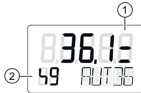
Figure 8-7 Display of a threshold 2 message: 2 bars means maintenance level "Maintenance demanded"
