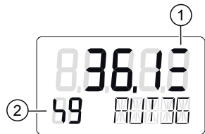
Figure 8-8 Display of a threshold 3 error message: 3 bars means maintenance level "Maintenance alarm"
