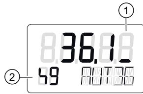
Figure 8-6 Display of a threshold 1 message: 1 bar means maintenance level "Maintenance required"
