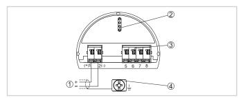
Secondary terminal connections (intrinsically safe devices)
