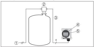
Fig. 2: Connection of VEGADIS 81 to the sensor
