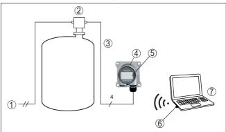
Fig. 6: Connection of VEGADIS 81 with Bluetooth to the sensor and connection to the PC
