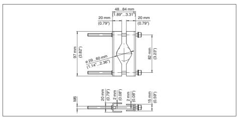
Fig. 34: Brackets for tube mounting of VEGADIS 81
