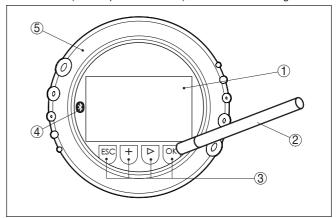
Fig. 24: Display and adjustment elements - with adjustment via magnetic pen
