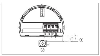
Fig. 14: Wiring plan VEGADIS 81 for 4 ... 20 mA/HART sensors
