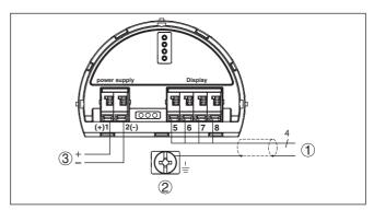
Fig. 15: Wiring plan VEGADIS 81 for 4 ... 20 mA/HART sensors, display and adjustment module with heating
