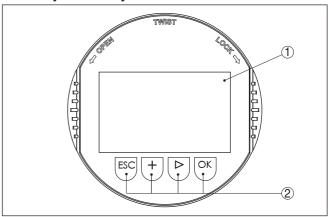
Fig. 23: Display and adjustment elements
