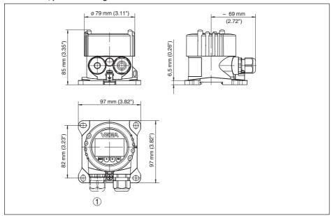
Fig. 30: VEGADIS 81 with plastic housing
