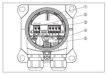
Fig. 13: Electronics and terminal compartment - VEGADIS 81 with heating
