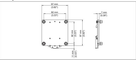
Fig. 33: Adapter plate for carrier rail mounting of VEGADIS 81
