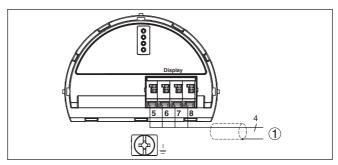
Fig. 16: Wiring plan VEGADIS 81 for PA/FF sensors
