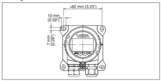
Fig. 7: Drilling dimensions for VEGADIS 81 for wall mounting
