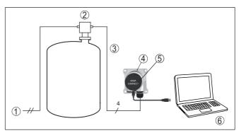
Fig. 5: Connection of VEGADIS 81 to the sensor and the PC
