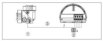
Fig. 20: Connection example 4 ... 20 mA/HART - connection via M12 plug connector and ready-made cable
