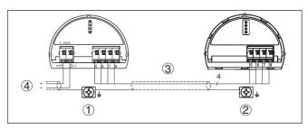
Fig. 19: Connection example 4 ... 20 mA/HART - connection via standard cable - screened
