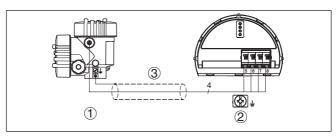
Fig. 21: Connection example Profibus PA, Foundation Fieldbus - Connection via M12 plug connector and open cable end
