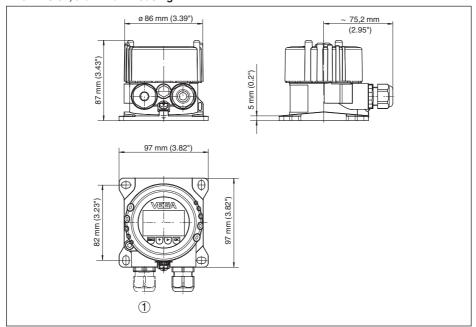
Fig. 31: VEGADIS 81 with Aluminium housing
