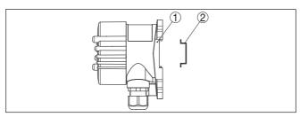
Fig. 8: VEGADIS 81 with plastic housing for carrier rail mounting
