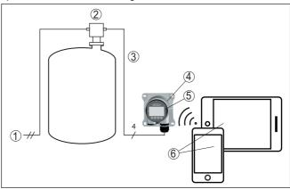
Fig. 4: Connection of VEGADIS 81 to the sensor
