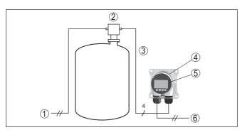
Fig. 3: Connection of VEGADIS 81 with heating to the sensor
