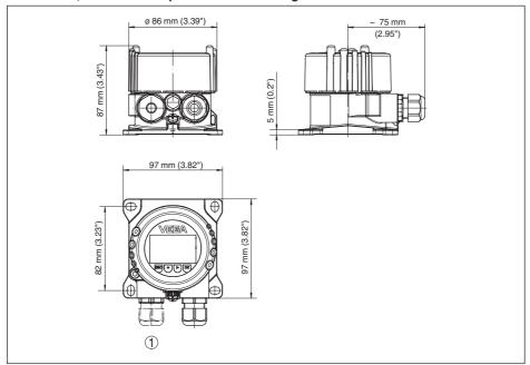
Fig. 32: VEGADIS 81 with stainless steel, precision cast housing
