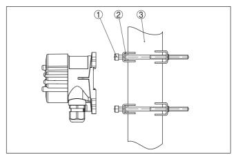
Fig. 10: VEGADIS 81 for tube mounting
