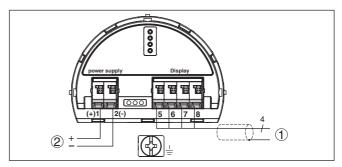
Fig. 17: Wiring plan VEGADIS 81 for PA/FF sensors, display and adjustment module with heating
