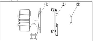
Fig. 9: VEGADIS 81 with aluminium and stainless steel housing for carrier rail mounting
