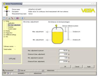
Fig. 27: Example of a DTM view
