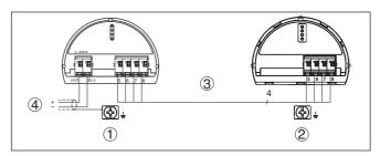
Fig. 18: Connection example 4 ... 20 mA/HART - connection via standard cable
