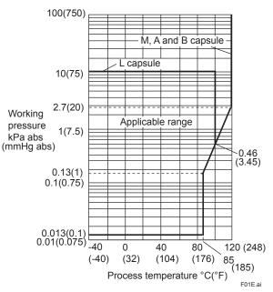
Figure 1. Working Pressure and Process Temperature
