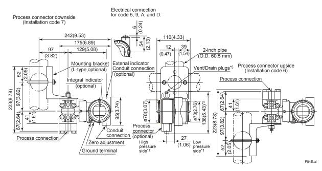
• Horizontal Impulse Piping Type (Installation code 9)
