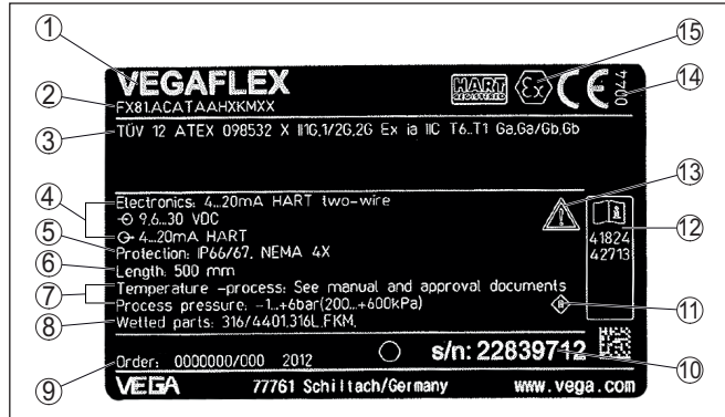
Fig. 1: Layout of the type label (example)
