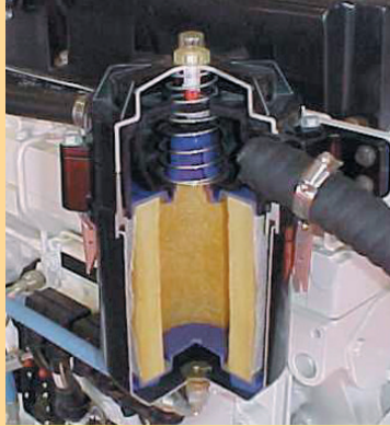
Cummins QSM11 marine engine with CCV cutaway
